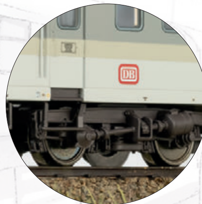
The type Dm 903 with type Minden-Deutz heavy trucks with double brake shoes, here Truck 2 with a type D150 axle generator on the right side of the car
