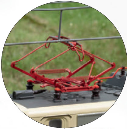
Newly designed type DBS 54 pantographs can be raised and lowered digitally
